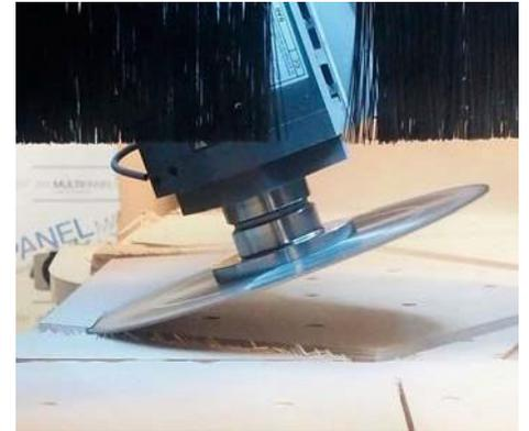
*/ Spectacular: The saw blade is also used as part of the nesting process on the Format-4-CNC machine.*
