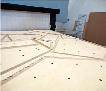
*/ The new nesting process saves up to 15% in material compared with the former process.*
