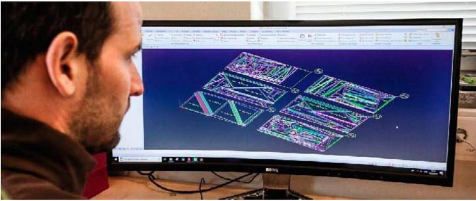
*I The CAD/CAM system Alphacam is the paramount software tool. Its high-performance nesting tool optimizes the arrangement of the many individual parts in the panels and generates all required CNC programs.*
