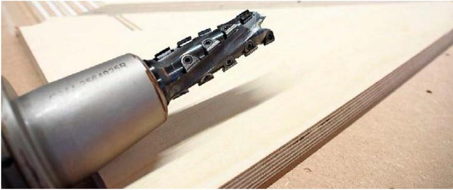
*/ High performance, easy handling: The Konstantin Mini from Aigner has a diameter of 25 mm. The 23 slide cutting edges can be changed by the user himself, drilling and circumferential cutting edges are identical.*
